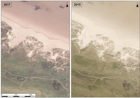
Figure 17 – Damage to dunes along Coatham Sands in 2017 (left) and 2015 (right)
